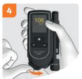
Testing is completed after approx. 5 seconds. Read the test result and close the tip over. The meter turns off.
