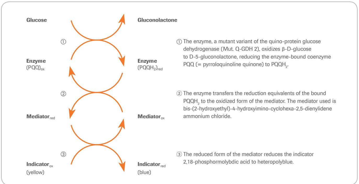
Figure 5: Determination reaction in the reactive film of the test area
