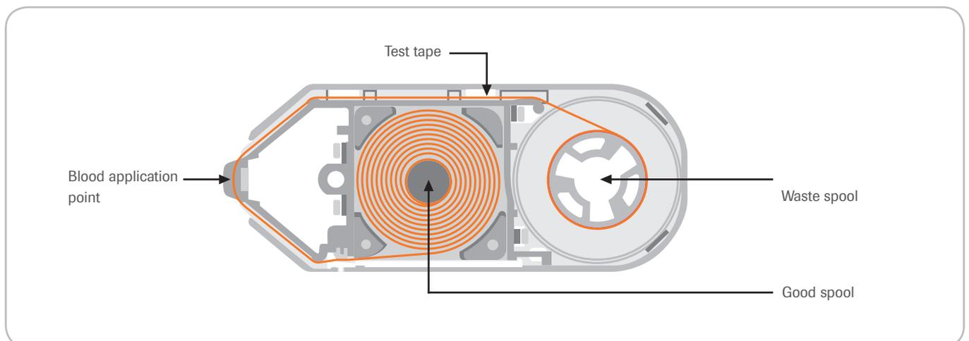
Figure 3: Schematic drawing of the Accu-Chek Mobile test cassette
