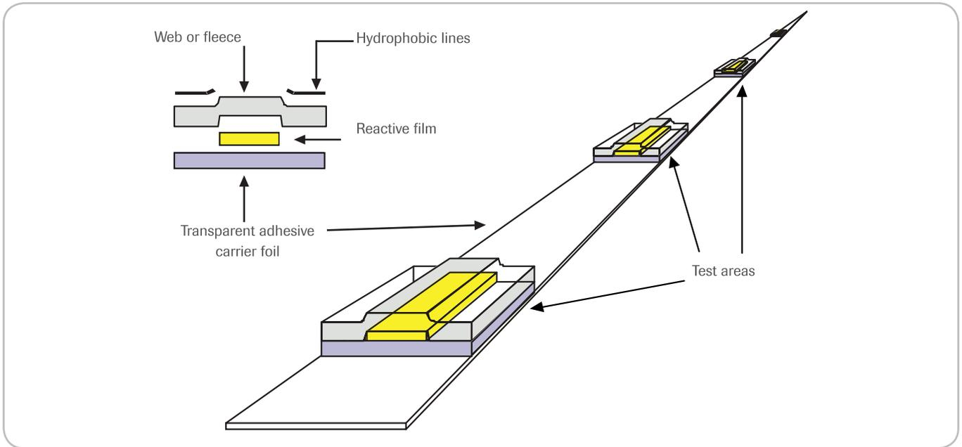
Figure 4: Schematic drawing of the Accu-Chek Mobile test tape
